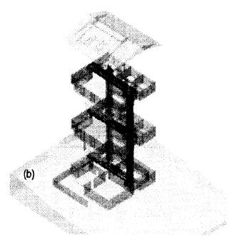
Fig. 3: (a) Exploded view of house and (b) core chases and shafts for wiring
