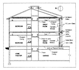
Fig. 4: North-south section through double envelope
