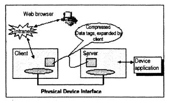
Fig. 6: Embedded device with browser access through client.
